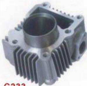
C233 CRYPTON Bore:49/51/54mm
